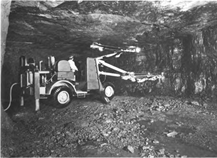
FIGURE 4 Modern mining machinery—A drill jumbo in use at St. Joseph Lead Company in Missouri. This unit is manufactured in the United States, based on a concept developed in Germany. The rotary-percussion drills mounted on the machine are capable of approximately twice the penetration rate of conventional pneumatic rock drills. About 500 tons of ore can be drilled per shift. (Photo courtesy John Reed.)
