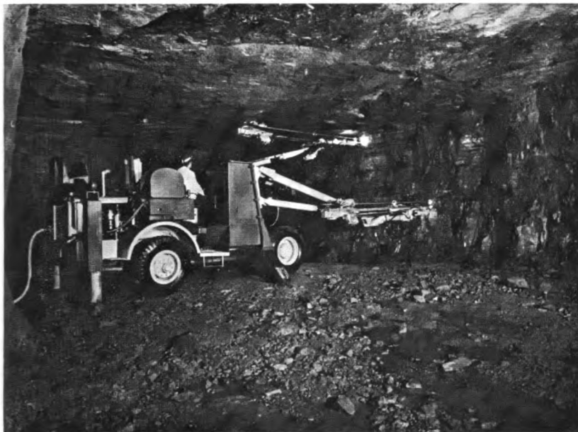
FIGURE 18 Two-man production jumbo mounting three pneumatic rock drills.
