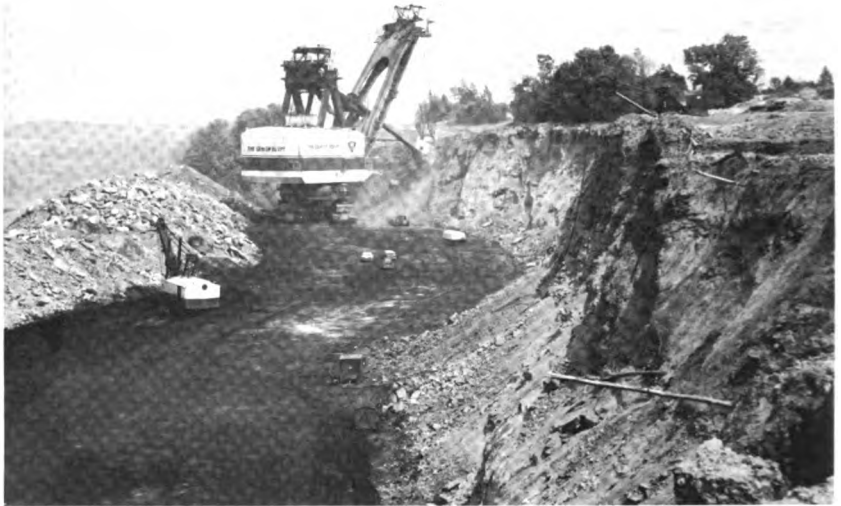
FIGURE 8 A large stripping shovel removing blasted overburden with a 130 cubic yard bucket. Coal loading shovel is in left foreground. Note relative size of cars in center on top of coal seam. Overburden in this case is only medium thick.
