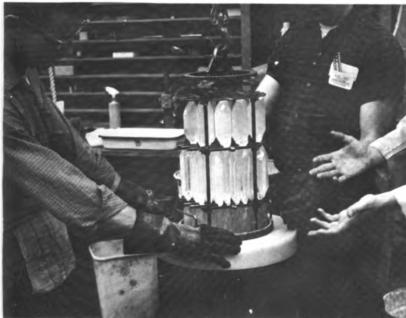
FIGURE 8 Synthetic quartz crystals grown at high pressure.
