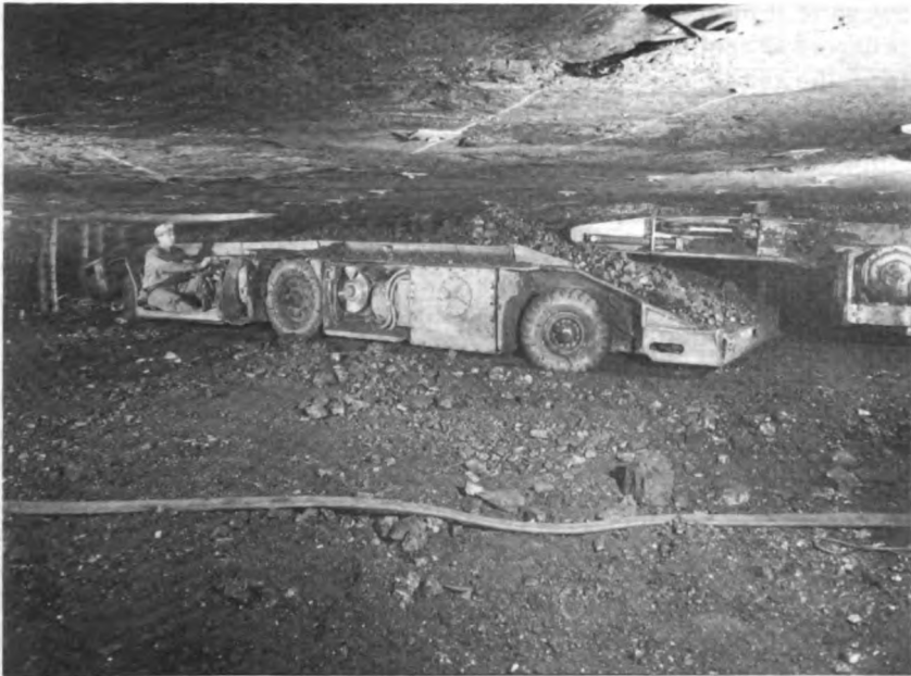
FIGURE 16 Shuttle car and loader under bolted roof in a medium thick coal seam.
