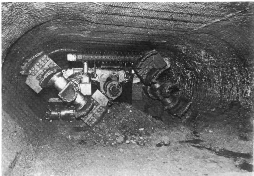
FIGURE 13 Boring type continuous miner trammed back from the coal face to show cutting tools.
