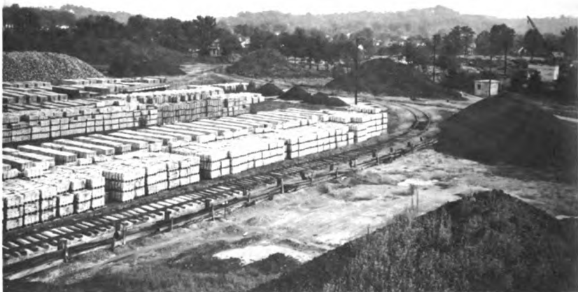
FIGURE 9 Open storage of several different metals and ores at one of the national stockpile depots. Materials are stored as close as possible to consumers to aid continuity of production despite disruption of transportation facilities in wartime. Note that provision is made for ready access by both truck and rail. As much as 1 million tons of ore may be stored in one pile, or in some cases, as little as 20 tons. (Photo courtesy U.S. Bureau of Mines, U.S. Department of the Interior.)
